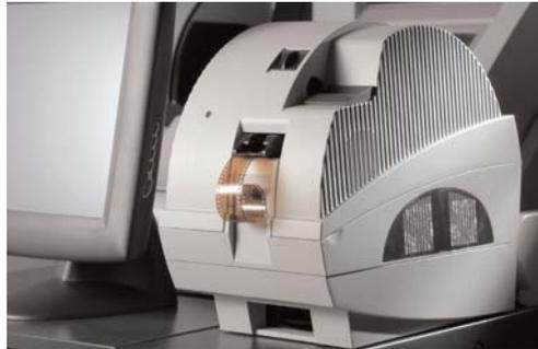
In addition, the standard Digital ICE™ software is automatically applied to remove undesired dust and scratches on the film. This technology uses infrared light to pinpoint any elements of dust and scratches and automatically corrects them by extrapolating image data from the surrounding area.
